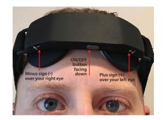
LIFTID is centered and electrodes are at the same height and straight
